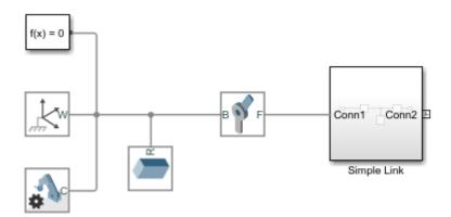
6 In the Solid block dialog box, specify the following parameters. This block connects rigidly to the World frame and therefore has no effect on model dynamics. You can leave the inertia parameters in their default values.
