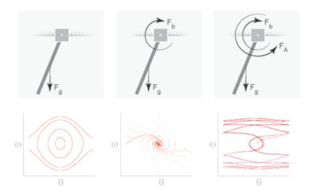
First, create the simple pendulum model in "Model a Simple Pendulum" on page 1-15. By adding forces and torques to this model, you incrementally change the pendulum from undamped and free to damped and driven. The forces and torques that you apply include:
