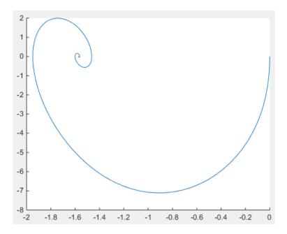
Try simulating the model using different starting angles. In the **Z Revolute Primitive (Rz)** > **State Targets** section, under **Specify Position Target**, specify **Value** parameter of the Revolute Joint block dialog box. The figure shows a compound phase plot for starting angles of -240, -180, -120, -60, 0, and 60 degrees.
