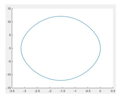
Try simulating the model using different starting angles. In the **Z Revolute Primitive (Rz)** > **State Targets** section, under **Specify Position Target**, specify the **Value** parameter of the Revolute Joint block dialog box. This figure shows a compound phase plot for starting angles of -80, -40, 0, 40, and 80 degrees.
