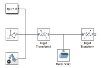
7 In the Brick Solid dialog box, specify the following parameters. These parameters define the simple link's physical properties, such as shape, mass, and appearance.
